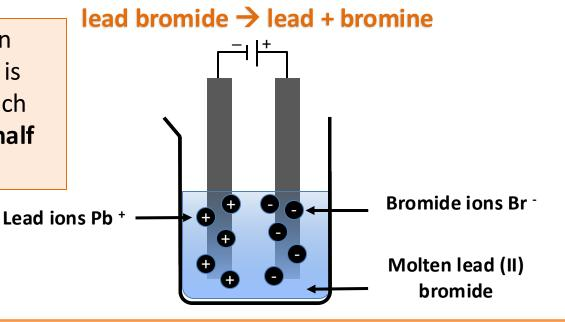
The positively charged lead ions Pb + (cations) are attracted to cathode and the negatively charged bromide ions Br - are attracted to the anode.
