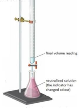
3. Stop adding the acid when the end-point is reached (the appropriate colour change in the indicator happens). Note the final volume reading. Repeat steps 1 to 3 until you get consistent readings.
