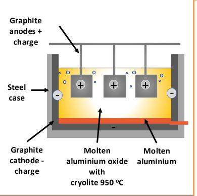
Aluminium oxide has a very **high melting point** so is mixed with molten **cryolite** to lower the temperature required to carry out the electrolysis. Aluminium goes to the negative electrode and sinks to bottom.
